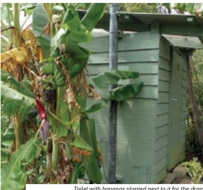
Toilet with bananas planted next to it for the drain
