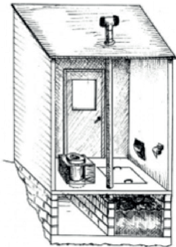
Two examples of compost toilet construction using the double chamber as a base
