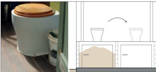
A stand-alone, commercial pedestal can be used, and then moved across for use on the other chamber to avoid having to buy two pedestals.
