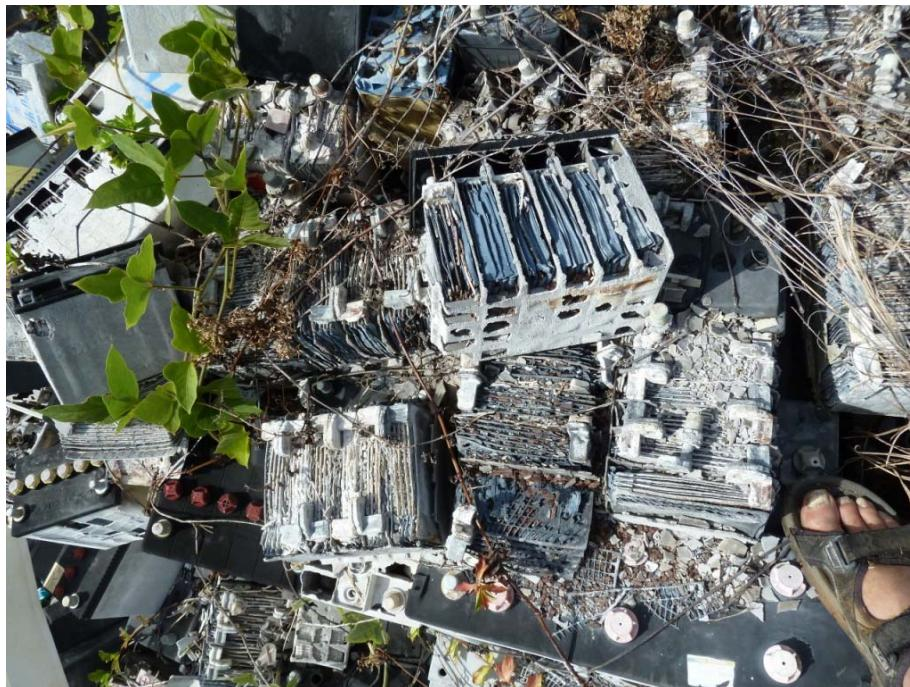
**Fig 12: ULABs in the Wallis stockpile that are severely sun damaged by long-term exposure in the stockpile. These may need additional packing materials to adequately pack them.**
